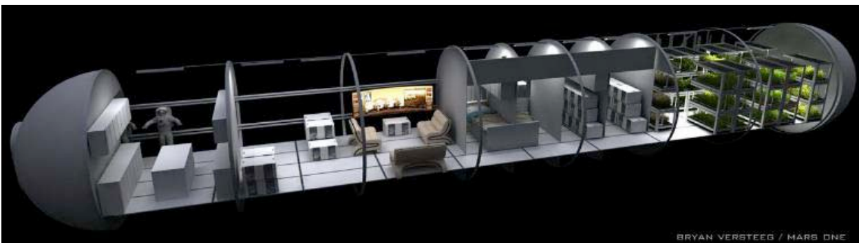
FIGURE 8. Longitudinal, cutaway view of the MarsOne 500 m 3 habitation and plant growth inflatable module. Credit: Bryan Versteed, MarsOne.
