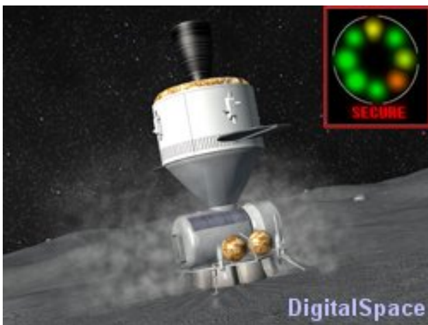
FIGURE 4b. Orion with mission/lander module makes a touchdown on the surface of an asteroid, lofting dust in the process. The icon in the upper right corner represents a symbology for safety status.
