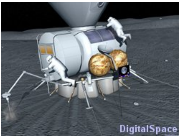
FIGURE 4c. EVA crewmembers translating around the mission/lander module while its robot arm drills into the regolith. This mission module would include an EVA airlock. Notice the landing blast pattern in the asteroidal dust.
