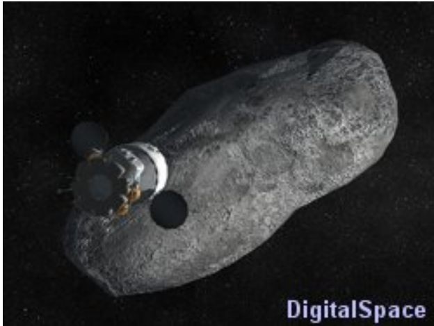
FIGURE 4a. Orion with a mission/lander module approaches a generic asteroid. The white Service Module is oversized compared to the LEO version so that it can carry the greater quantity of propellant and consumables to support the crew throughout the longer mission.
